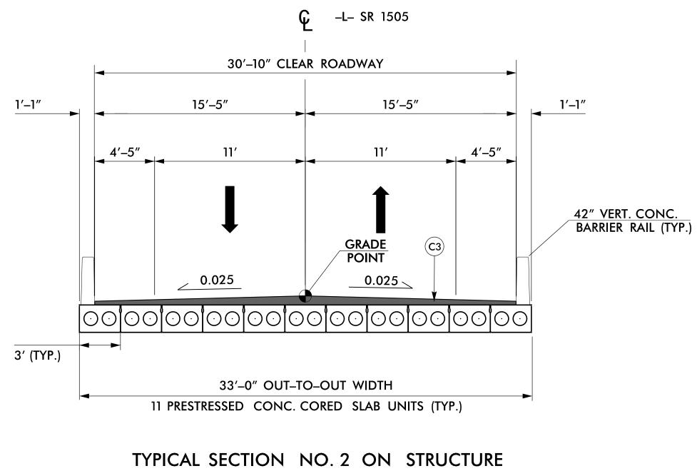
BRIDGE 650015 OVER WILDCAT CREEK –L– STA. 15+03.35 TO STA. 16+10.72 \*\* SEE STRUCTURES PLANS FOR AWS THICKNESS
