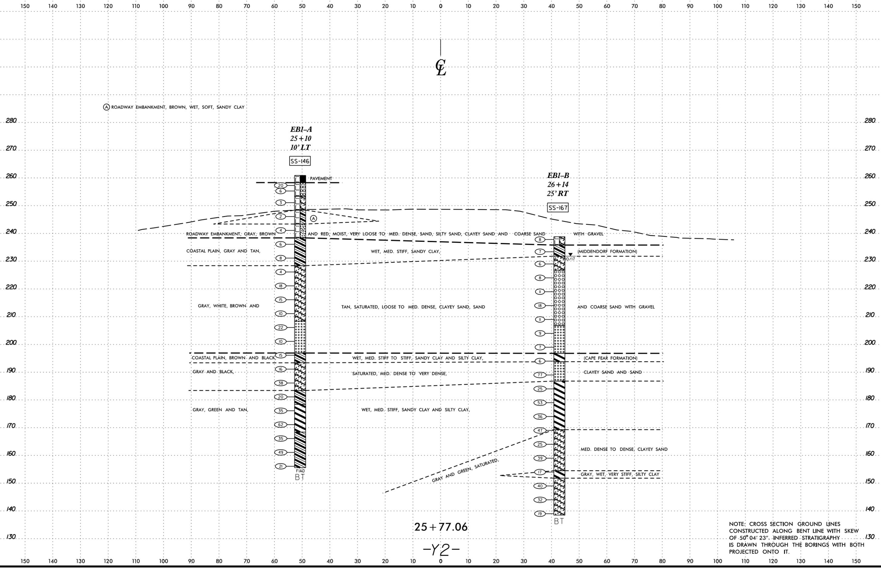
NOTE: CROSS SECTION GROUND LINES CONSTRUCTED ALONG BENT LINE WITH SKEW OF 50° 04' 23". INFERRED STRATIGRAPHY IS DRAWN THROUGH THE BORINGS WITH BOTH PROJECTED ONTO IT.
