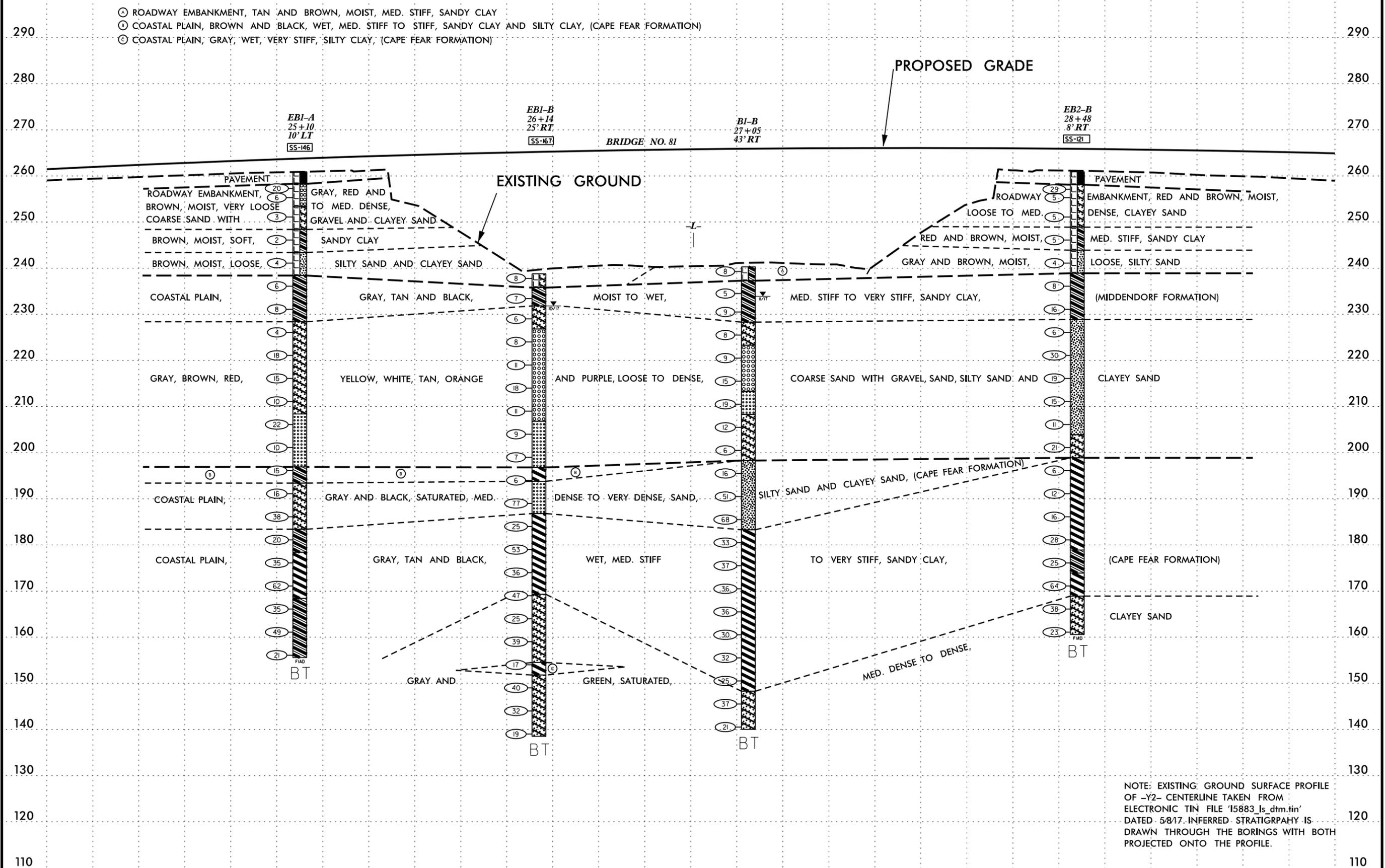
NOTE: EXISTING GROUND SURFACE PROFILE OF -Y2- CENTERLINE TAKEN FROM ELECTRONIC TIN FILE 'I5883\_Is\_dtm.tin' DATED 5/8/17. INFERRED STRATIGRAPHY IS DRAWN THROUGH THE BORINGS WITH BOTH PROJECTED ONTO THE PROFILE.
