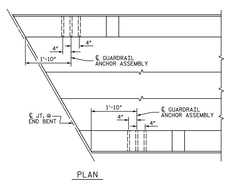
LOCATION OF GUARDRAIL ANCHOR AT END POST
