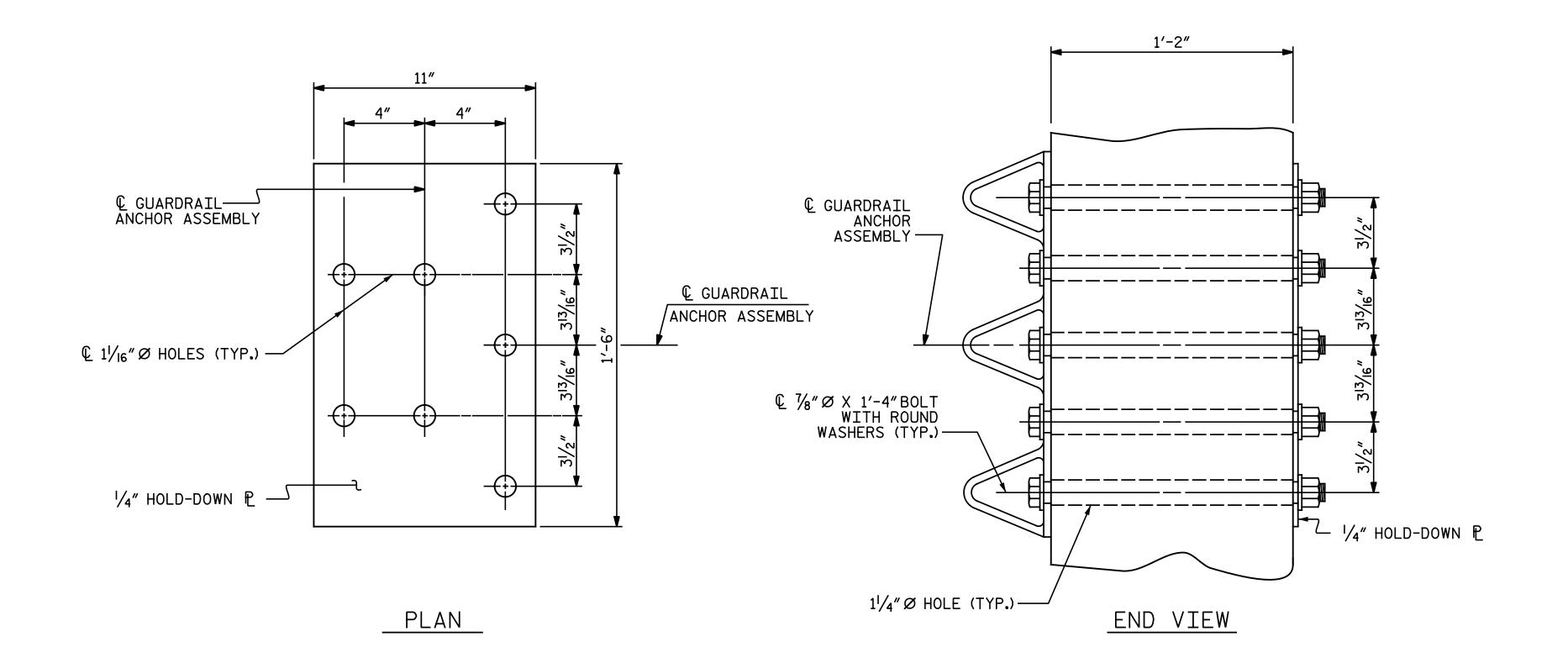
GUARDRAIL ANCHOR ASSEMBLY DETAILS
