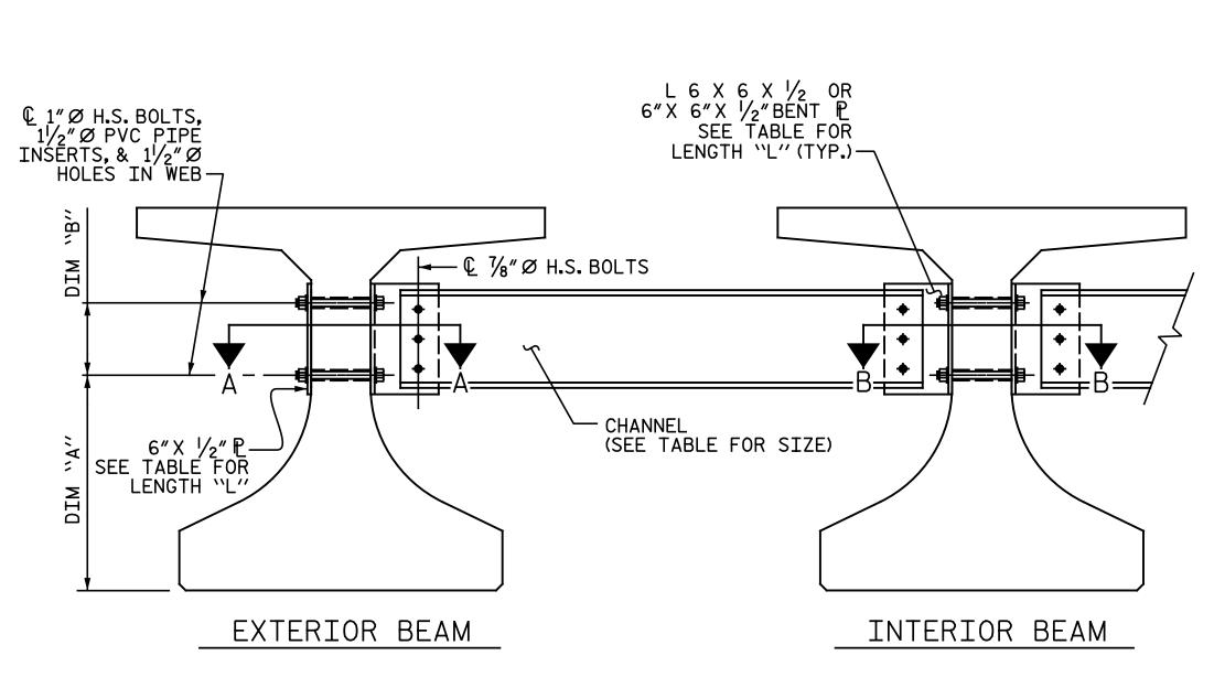
PART SECTION AT INTERMEDIATE DIAPHRAGM
