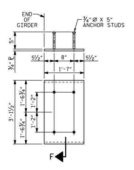
EMBEDDED PLATE "B-1" DETAILS FOR 54", 72", & 78" CFRP F.I.B.
