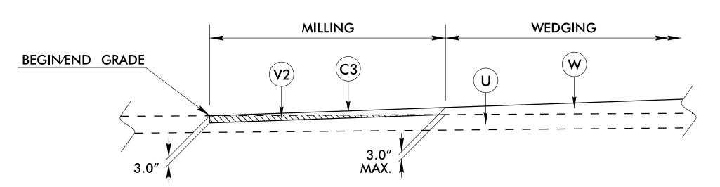
DETAIL OF 0" - 3" MILLING AT PAVEMENT TIE-INS
