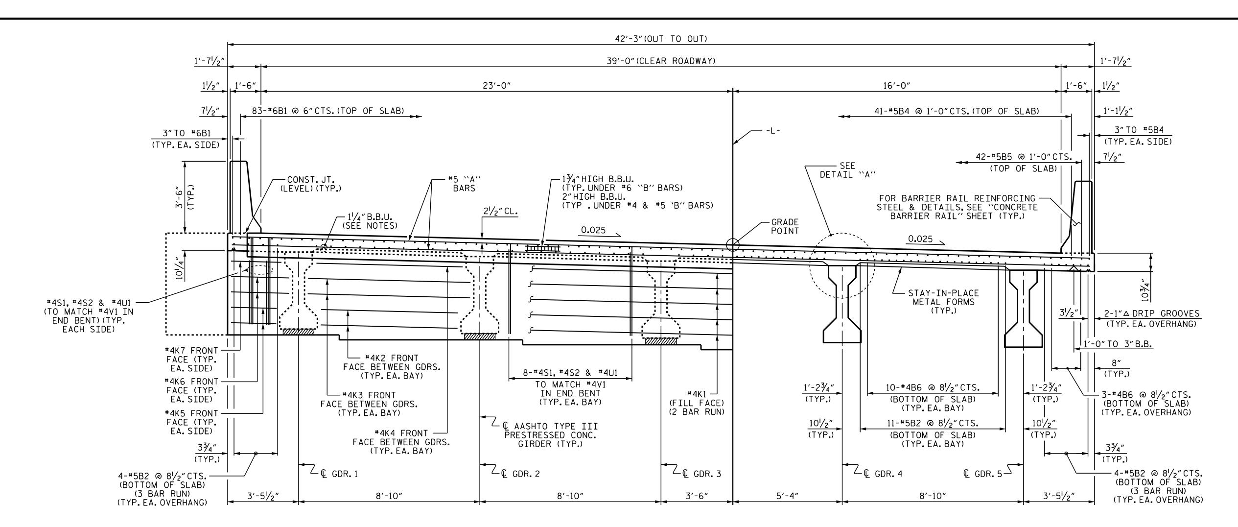
PART SECTION - INTEGRAL END BENT DIAPHRAGM
