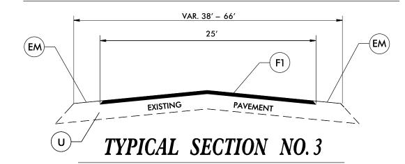
NOTE: TYPE III MICROSURFACING TO BE PLACED BETWEEN MILLED RUMBLE STRIPS AND GORE AREAS ONLY.
