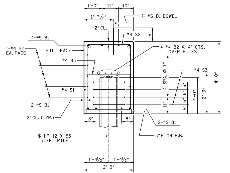
SECTION A-A (CONCRETE COLLAR NOT SHOWN FOR CLARITY. SEE "CORROSION PROTECTION FOR STEEL PILES DETAIL.") PLANS PREPARED BY: NGINEERS ASSOCIATES
