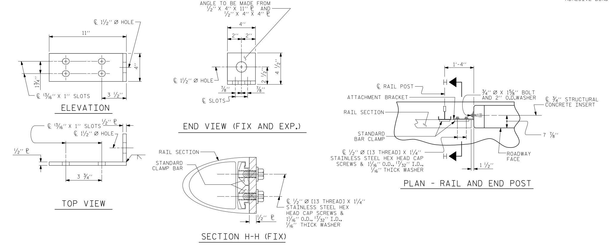
DETAILS FOR ATTACHING METAL RAIL TO END POST
