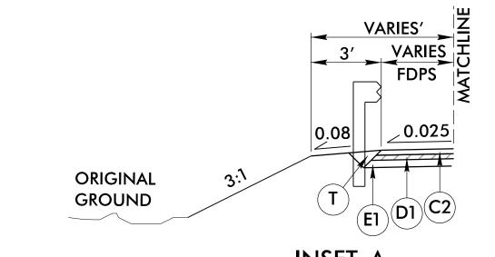
INSET A (USE WITH TYPICAL SECTIONS NO. 1 & 2) USE IN GUARDRAIL LOCATIONS (SEE GUARDRAIL SUMMARY 3B-1)
