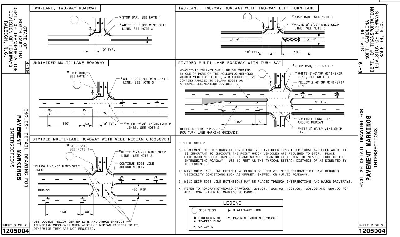
REVISED PAVEMENT MARKING ROADWAY STANDARD DRAWING
