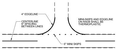
NOTE: MINI SKIPS SHALL BE PLACED ON A 8' CYCLE, CONTAINING A 6' AND 2' SKIP, THE WIDTH OF THE SKIP SHALL BE 6".
