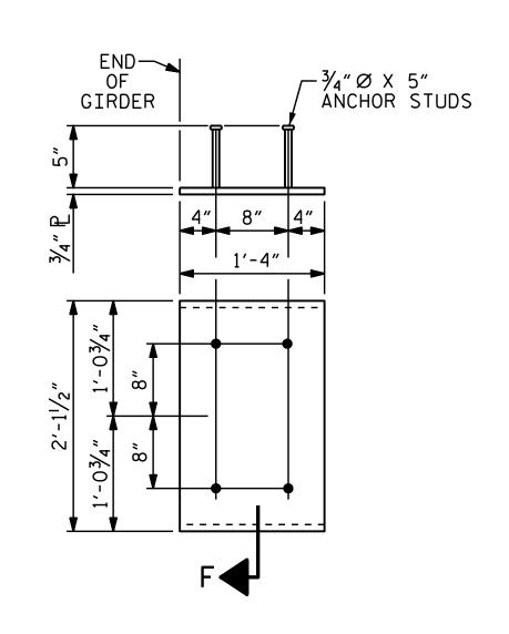
EMBEDDED PLATE "B-1" DETAILS FOR AASHTO TYPE IV GIRDER AND 72" MODIFIED BULB TEES
