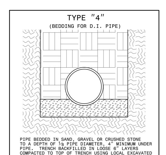
MATERIAL, IF APPROVED BY THE ENGINEER, OR SELECT MATERIAL. ALL MATERIAL SHALL BE FREE OF ROCKS, FOREIGN MATERIAL, AND FROZEN EARTH. COMPACTION SHALL BE TO APPROX. 95% DENSITY IN ACCORDANCE
