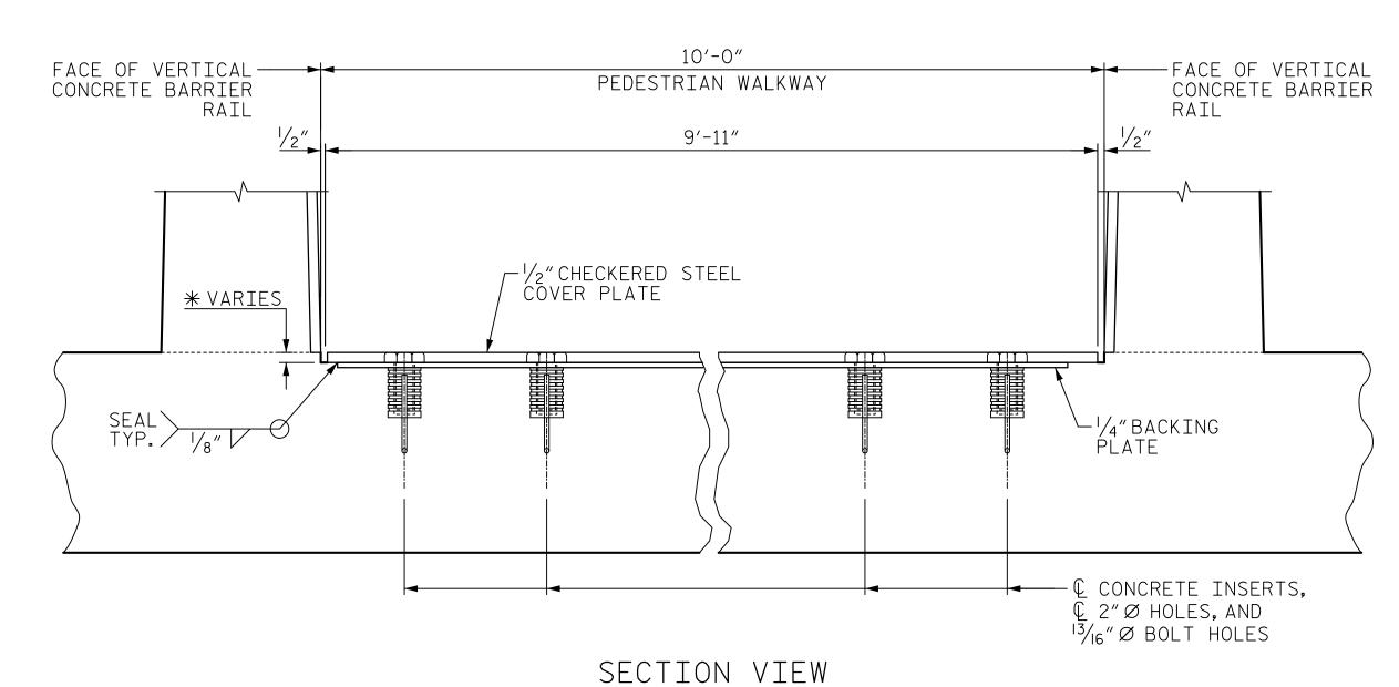
\*  $^{13}/_{16}$ " FOR SIDE OF JOINT HAVING THE  $^{12}$ " COVER PLATE WITH  $^{14}$ " BACKING PLATE.  $^{9}/_{16}$ " FOR SIDE OF JOINT HAVING ONLY THE  $^{12}/_{2}$ " COVER PLATE.
