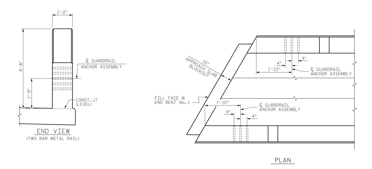
LOCATION OF GUARDRAIL ANCHOR AT END POST
