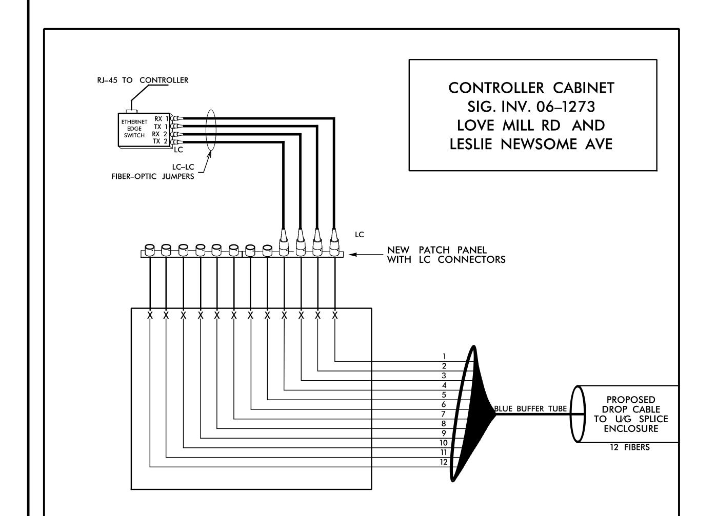
LEGEND COLOR CODE X = FUSION SPLICE INDIVIDUAL FIBER TIA/EIA 598-A (7) RED (1) BLUE C = CAP AND SEAL(2) ORANGE (8) BLACK EXPRESS ENTIRE BUFFER TUBE /FIBERS **EXPRESS** (3) GREEN (9) YELLOW THROUGH WITHOUT CUTTING (4) BROWN (10) VIOLET (11) ROSE SPLICE ALL FIBERS IN BUFFER (5) SLATE BUFFER SPLICE = TUBE COLOR TO COLOR (6) WHITE (12) AQUA
