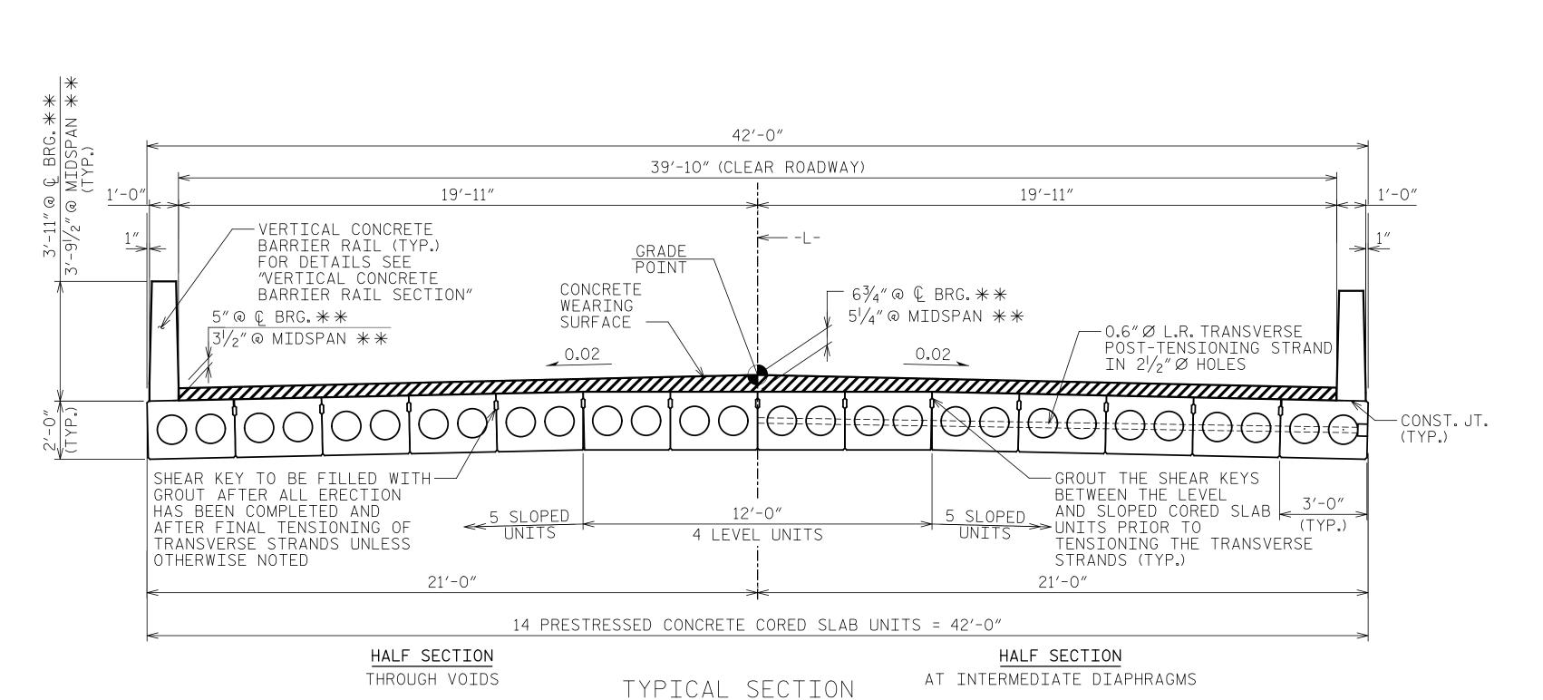
\*\* BASED ON PREDICTED FINAL CAMBER AND THEORETICAL GRADE LINE ELEVATIONS. THE CONCRETE WEARING SURFACE THICKNESS AND HEIGHT OF THE BARRIER RAIL VARIES WHILE THE TOP OF THE BARRIER RAIL FOLLOWS THE PROFILE OF THE GUTTERLINE.
