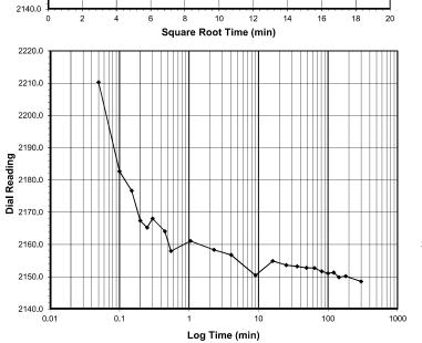
**Test Load** (tsf) 4.0-1.0 Final Reading (div) 2148.5 Consolidometer No. R470 0.0001 1 Division
