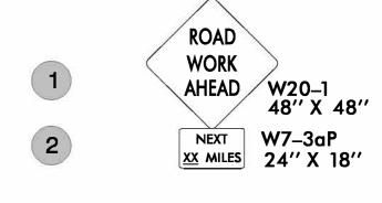
PLACE 1000' PRIOR TO BEGINNING OF CONSTRUCTION LIMITS. ONLY USED ON -Y- LINES IF RESURFACING LIMITS EXTEND 1000' ALONG -Y- LINE.
