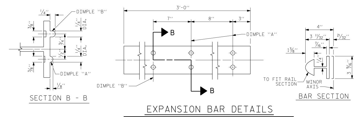
$/_2$ " Ø [13 THREAD] HOLE FOR  $/_2$ " Ø X 1" STAINLESS STEEL HEX HEAD CAP SCREW &  $1/_{16}$ " O.D.,  $17/_{32}$ " I.D.,  $-/_{16}$ " THICK WASHER (TYP.)
