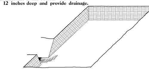
3. Backfill the trench with 2 inches well rotted sawdust. Place a 2 inch layer of well rotted sawdust at a sloping angle
