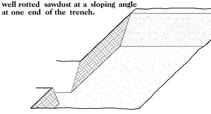
4. Place a single layer of plants against the sloping end so that the root collar is at ground level.
