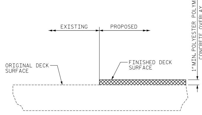
DETAIL FOR POLYESTER POLYMER CONCRETE OVERLAY
