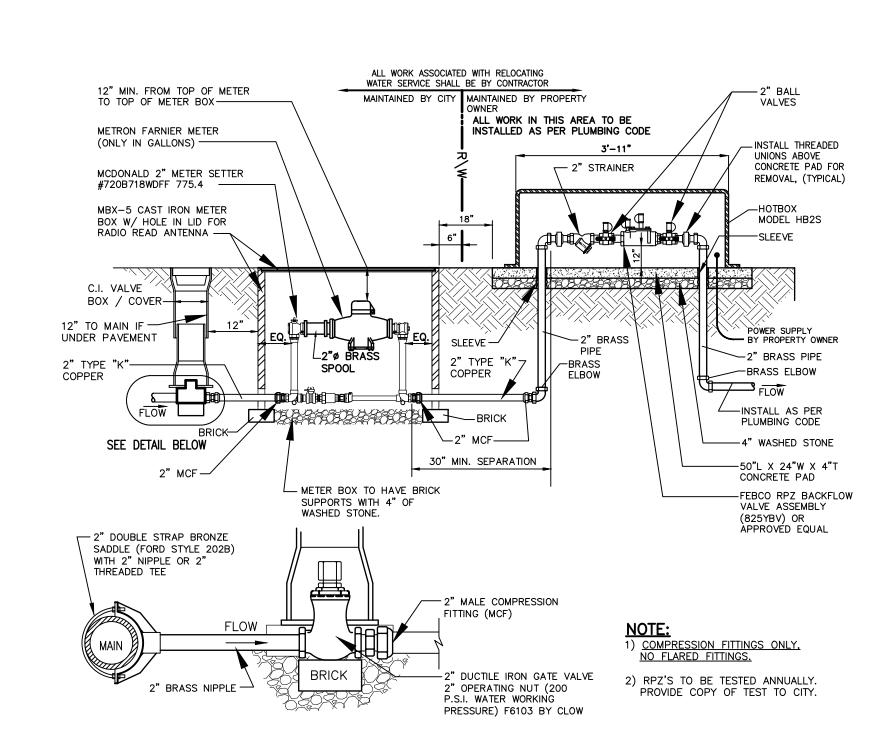
2" WATER CONNECTION WITH RPZ BACKFLOW ASSEMBLY
