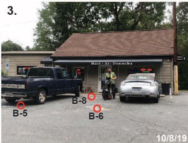
Collecting GPR data at Parcel #008. Red circles show location of soil borings B-5, B-6 and B-8 where contaminated soil was documented.
