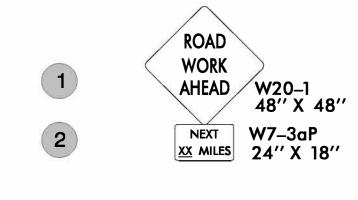
PLACE 1000' PRIOR TO BEGINNING OF CONSTRUCTION LIMITS. ONLY USED ON -Y- LINES IF RESURFACING LIMITS EXTEND 1000' ALONG -Y- LINE.
