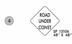
THESE ARE FOR -Y- LINES THAT ARE "THROUGH" ROADWAYS. DEAD END AND SUBDIVISION ROADS ARE NOT "THROUGH" ROADWAYS. INSTALL 500' +/- FROM EACH -Y- LINE APPROACH AS SHOWN ABOVE. FOR MULTIPLE -Y- LINES THAT ARE SEPARATED BY 0.25 MILES OR LESS, TREAT AS A SINGLE UNIT AND INSTALL WITHIN 500' OF EACH APPROACH. A MAXIMUM OF 2 SIGN SETS PER MILE. DO NOT SP 13106 48" X 48" INSTALL WHEN -Y- LINES ARE WITHIN 0.5 MILES FROM "END ROAD WORK" SIGN.
