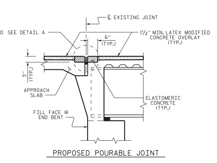
JOINT INSTALLATION SEQUENCE AT END BENTS (SECTION A-A)
