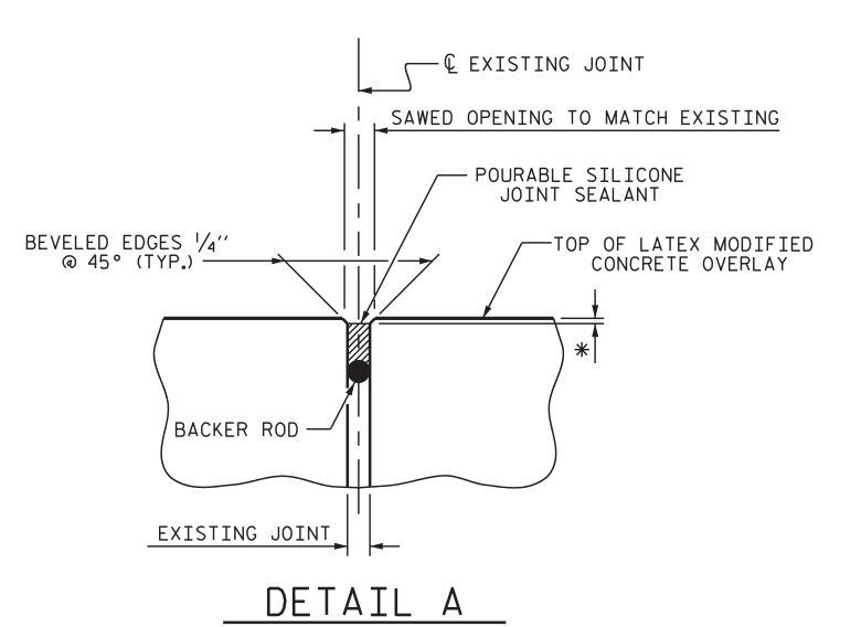
\* POURABLE SILICONE JOINT SEALANT SHALL BE RECESSED AS PER MANUFACTURER'S RECOMMENDATIONS.
