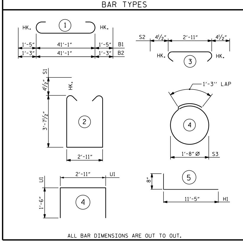
INTEGRAL END BENT #2 NO. SIZE TYPE LENGTH WEIGHT **#**10 43'-11" 756 B1 #9 43′-7″ 741 B2 #5 STR 41′-3″ 430 B3 10 #4 STR 21'-10" #4 STR 2'-11" B5 21 #4 STR В6 7′-10″ 26 #4 STR 4'-10" 48 15 В7 50 #5 5 12'-1" 630 24 #5 STR 3'-9" 94 H2 50 | #4 | 2 | 10'-11" | 365 S1 50 #4 3 3′-8″ 122 S2 20 #4 4 6'-6" S3 87 18 | #4 | STR | 5'-11" U1 68 | #4 | STR | 6'-2" | 280 64 #4 STR 8'-10" 378 ٧2 64 #4 STR 8'-4" 356 REINFORCING STEEL = 4522 LBS CLASS A CONCRETE
