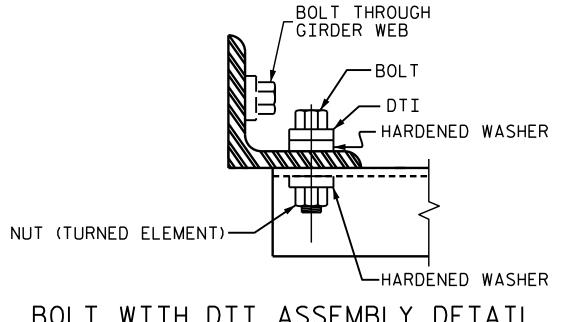
BOLT WITH DTI ASSEMBLY DETAIL
