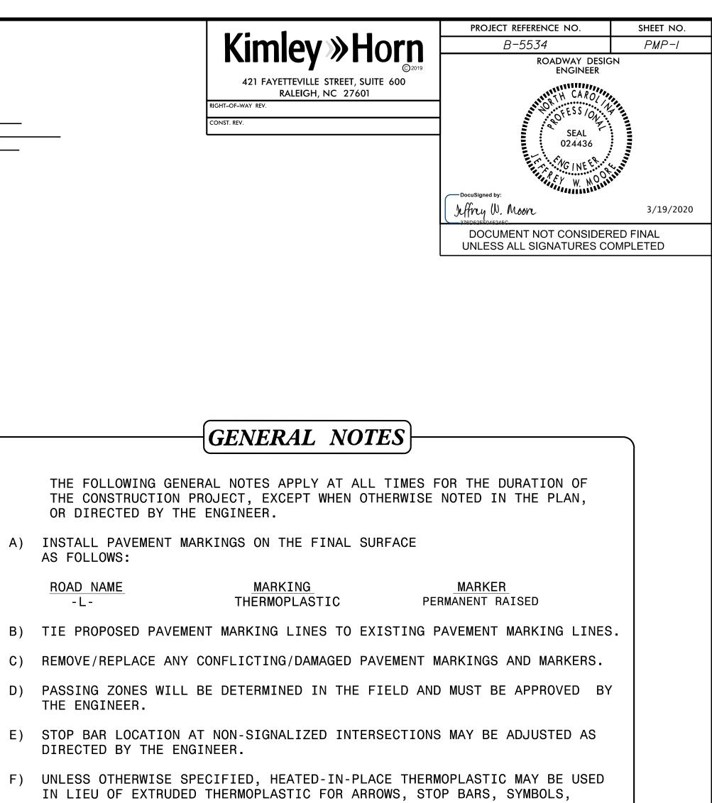
CHARACTERS AND DIAGONALS. IF HEATED-IN-PLACE IS USED, IT SHALL BE PAID FOR USING THE EXTRUDED THERMOPLASTIC PAY ITEM.
