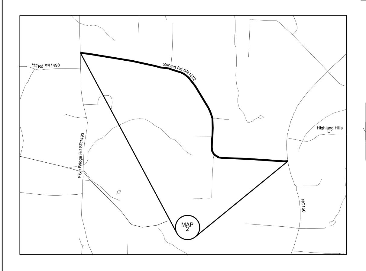
Map 2 Sunset Rd SR1522 From NC150 to Frye Bridge Rd SR1493 Mill 0-1 1/2" incidental mill beginning, end and at all SR intersections Pave 1 1/2" S9.5B
