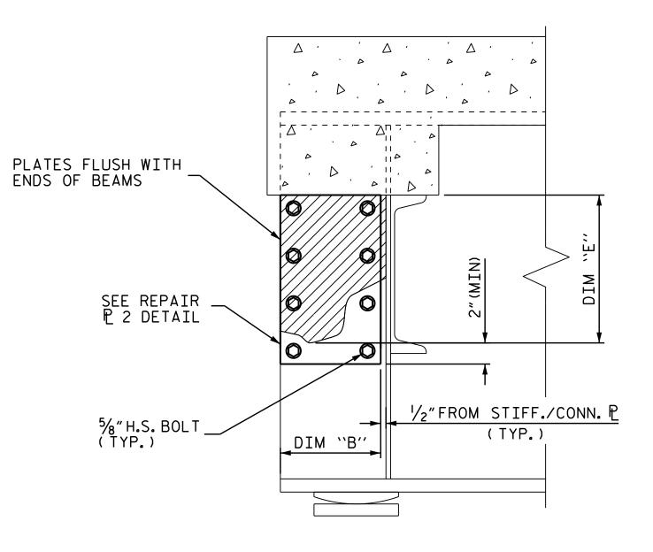
BEAM END SECTION LOSS PLATING REPAIR (DIMENSION ``E'' GREATER THAN  $6\frac{1}{2}$ " USE REPAIR  $\mathbb{P}(2)$ )
