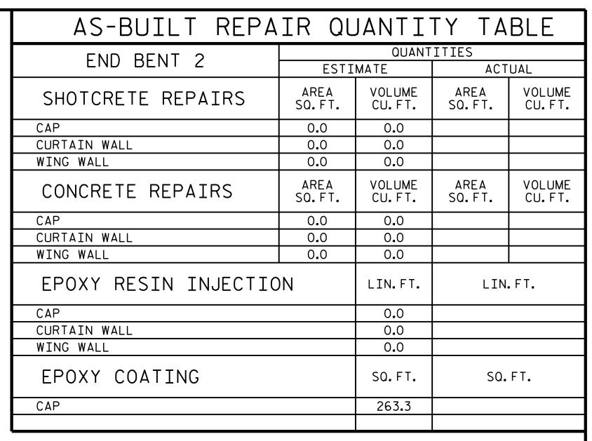
VALUES IN CHART REPRESENT ESTIMATED REPAIR TOTALS AFTER REMOVAL OF UNSOUND CONCRETE. MINIMUM OF 1"BEHIND REBAR AND MINIMUM 2"CLEARANCE TO SAWCUT. SEE "TYPICAL CAP AND COLUMN REPAIR DETAILS" SHEET.
