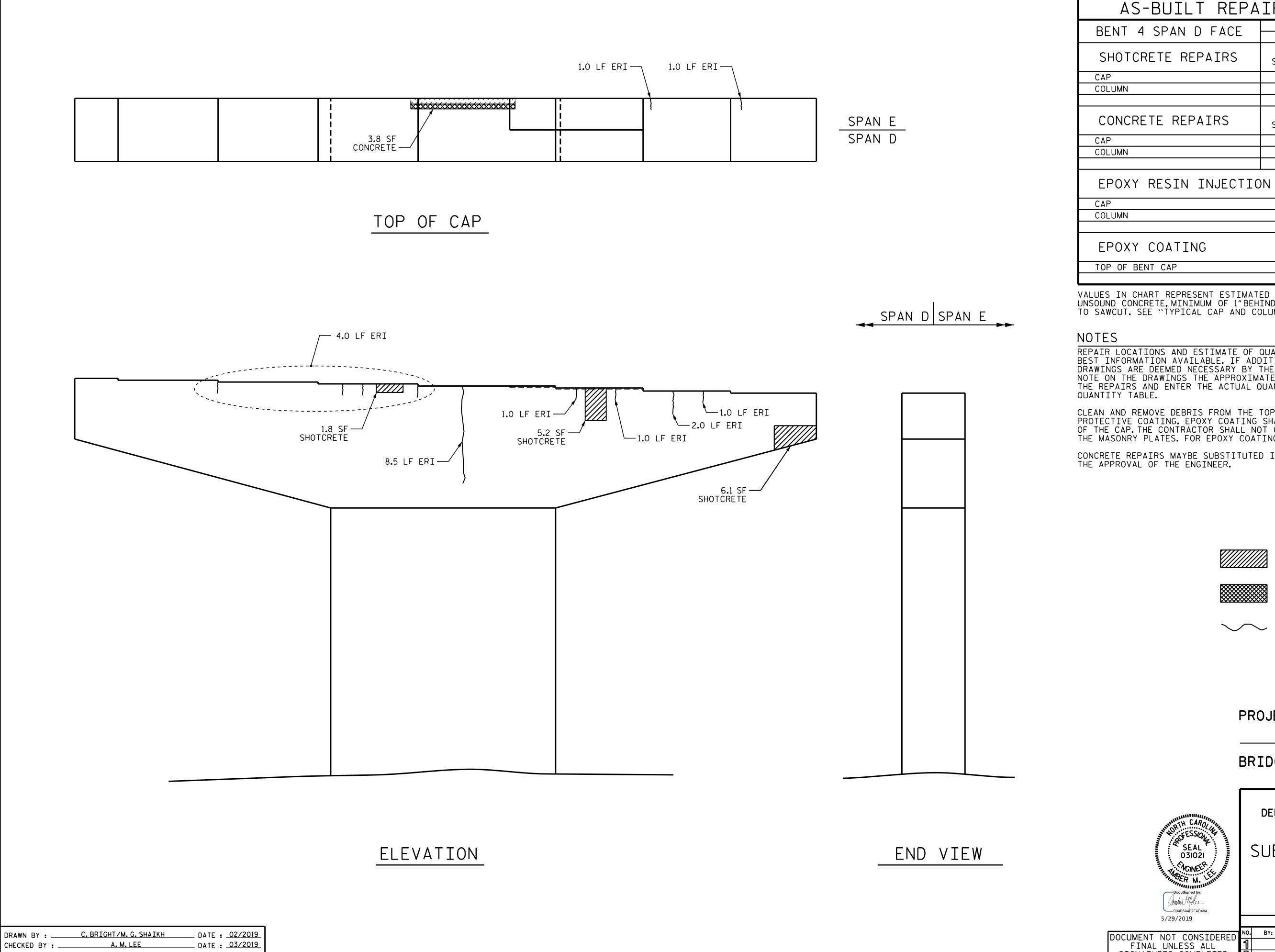
AS-BUILT REPAIR QUANTITY TABLE QUANTITIES ESTIMATE ACTUAL VOLUME CU.FT. VOLUME SQ. FT. SQ.FT. CU.FT. 13.1 6.6 0.0 0.0 AREA SQ.FT. VOLUME CU.FT. VOLUME SQ.FT. CU.FT. 3.8 1.9 0.0 0.0 LIN.FT. LIN.FT. 17.5 0.0 SQ.FT. SQ.FT. 355.0
