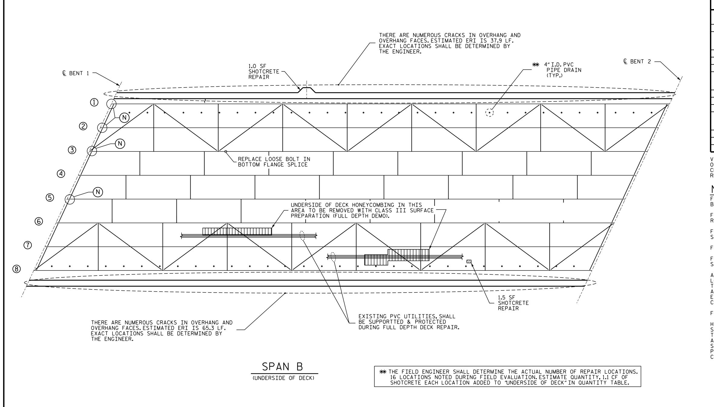
AS-BUILT REPAIR QUANTITY TABLE DECK UNDERSIDE REPAIRS - SPAN B ESTIMATE ACTUAL AREA VOLUME VOLUME SHOTCRETE REPAIRS CU.FT. SQ.FT. | SQ. FT. | CU. FT. UNDERSIDE OF DECK 17.6 7.3 CONCRETE DIAPHRAGM 0.0 0.0 OVERHANG 0.0 0.0 VOLUME CU.FT. AREA VOLUME CONCRETE REPAIRS SQ. FT. CU. FT. SQ.FT UNDERSIDE OF DECK 0.0 0.0 CONCRETE DIAPHRAGM 0.0 0.0 OVERHANG 0.0 0.0 EPOXY RESIN INJECTION LIN.FT. LIN.FT. UNDERSIDE OF DECK 0.0 CONCRETE DIAPHRAGM 0.0 OVERHANG 103.2
