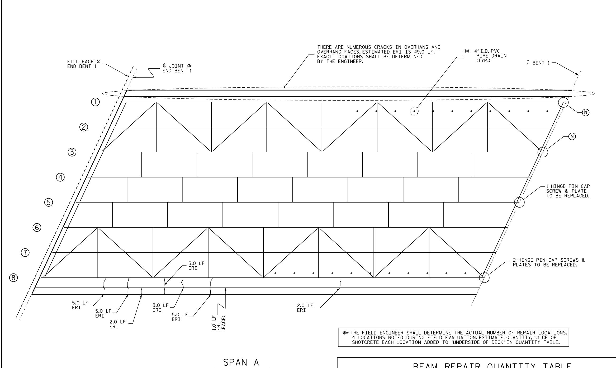
AS-BUILT REPAIR QUANTITY TABLE DECK UNDERSIDE REPAIRS - SPAN A ESTIMATE ACTUAL AREA VOLUME VOLUME SHOTCRETE REPAIRS CU.FT. SQ.FT. | SQ. FT. | CU. FT. UNDERSIDE OF DECK 4.4 1.8 CONCRETE DIAPHRAGM 0.0 0.0 OVERHANG 0.0 0.0 VOLUME CU.FT. AREA VOLUME CONCRETE REPAIRS SQ. FT. CU. FT. SQ.FT UNDERSIDE OF DECK 0.0 0.0 CONCRETE DIAPHRAGM 0.0 0.0 OVERHANG 0.0 0.0 EPOXY RESIN INJECTION LIN.FT. LIN.FT. UNDERSIDE OF DECK 0.0 CONCRETE DIAPHRAGM 0.0 OVERHANG 77.0
