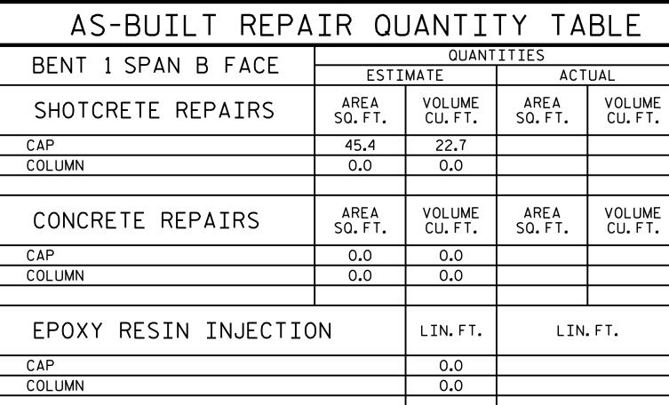
VALUES IN CHART REPRESENT ESTIMATED REPAIR TOTALS AFTER REMOVAL OF UNSOUND CONCRETE, MINIMUM OF 1"BEHIND REBAR AND MINIMUM 2"CLEARANCE TO SAWCUT. SEE "TYPICAL CAP AND COLUMN REPAIR DETAILS" SHEET.
