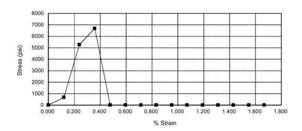
ASTM D-7012-10 METHOD C
