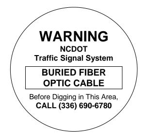
Overall Junction Box Marker Dimensions: 2.5" diameter Text: Black Background: Light Gray (to blend with concrete and granite surfaces)
