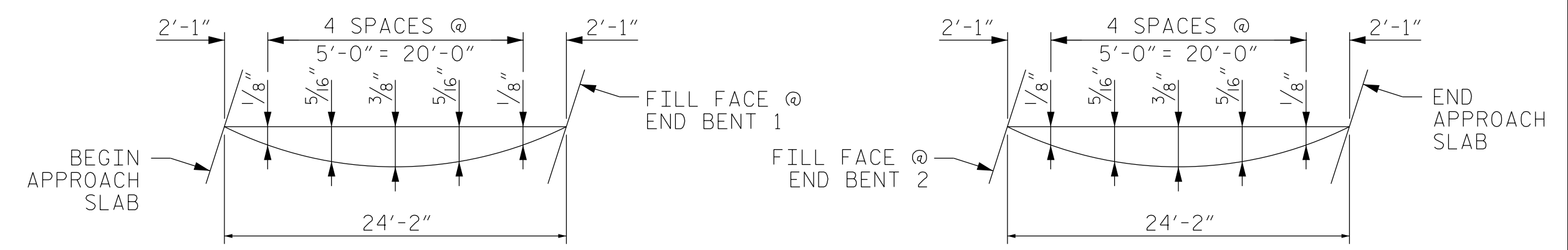
LEFT EDGE OF SLAB ARC OFFSETS APPROACH SLAB AT END BENT 1
