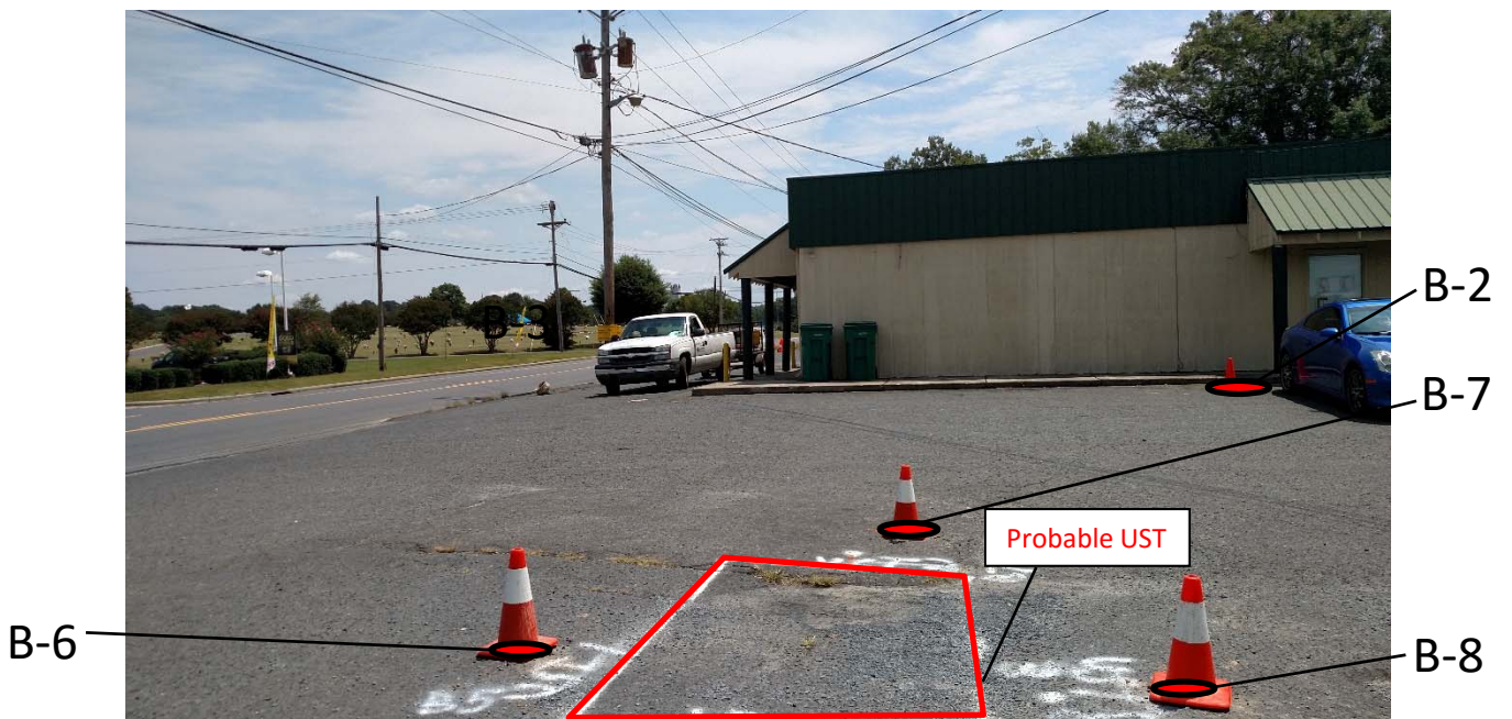
Photo #2: Boring locations B-2, B-6 through B-8, and a probable UST located west of the retail store front, facing southeast.
