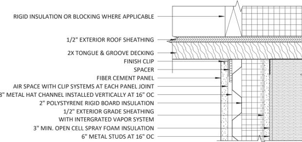
6 TYPICAL SOFFIT DETAIL @ NICHIBA
