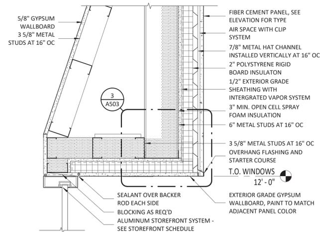
6 OVERHANG SOFFIT DETAIL @ ENTRY
