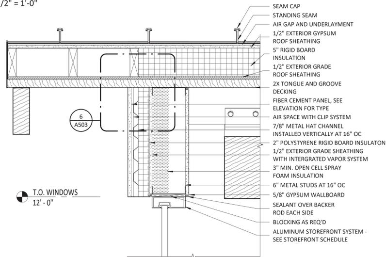
5 ROOF DETAIL @ REAR RAKE
