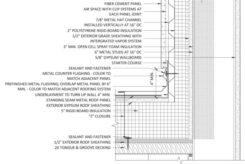
5 TYPICAL ROOF END WALL FLASHING DETAIL
