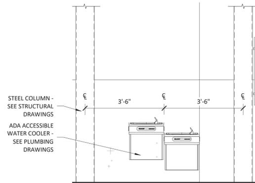
5 WATER COOLER ELEVATION
