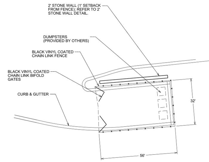
CHAIN LINK FENCE AND BIFOLD GATE
