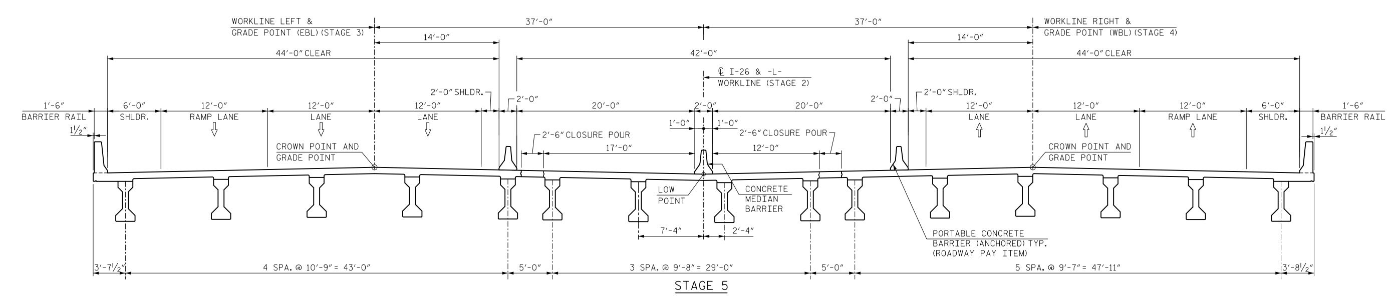
(PLACE SINGLE PORTABLE CONCRETE BARRIER, SHIFT TRAFFIC FROM MEDIAN BRIDGE SECTION TO NEW RIGHT LANE BRIDGE, REMOVE TWO PORTABLE CONCRETE BARRIERS (ANCHORED) IN MEDIAN BRIDGE SECTION. REMOVE TEMPORARY ASPHALT PAVEMENT ON BRIDGE, TIE STAGES TOGETHER WITH CLOSURE POURS, GROOVE BRIDGE FLOORS, BUILD CONCRETE MEDIAN BARRIER)
