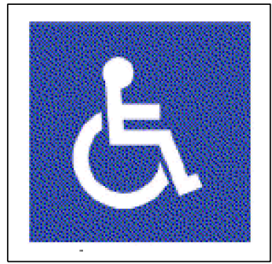
HEATED-IN-PLACE THERMOPLASTIC PAVEMENT MARKING SYMBOL FHWA/ADA APPROVED SYMBOL & BORDER: WHITE BACKGROUND: BLUE
