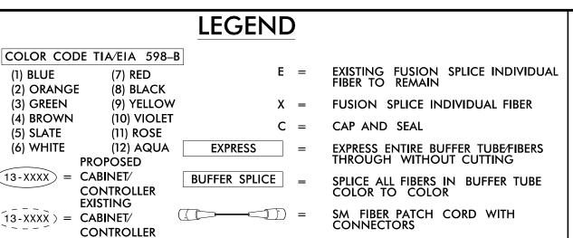
UNUSED FIBERS AND/OR BUFFER TUBES LEFT COILED AND STORED IN SPLICE TRAY.
