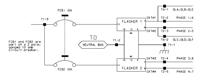
Ensure auxiliary output files are wired as follows:
